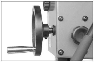
Figure 15. Guide post handwheel installed.
